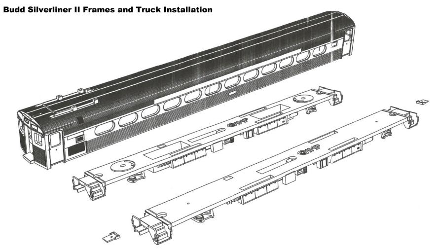
Note orientation of frame when installed in body. The frame is installed by means of three 2-56 screws (included with shell). Trucks are screwed in place on nonpowered frame. Drill bolster holes for 2-56 screws (not included). You'll need two 2-56 screws and two 2-56 washers to hold the trucks in place. Make sure the trucks can move freely and
