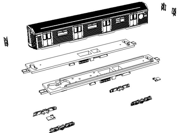
Use Bowser #125115 mechanism for powered cars. Use Bowser trailer trucks with 33" wheels for nonpowered cars. Truck sideframes fit Bowser trucks. Use 2/56 screws (included with body shells) to attach frame to body. Use 2-56 screws (not included) to attach coupler pockets. Paint Body Shell a bright silver paint (chrome or flaky metallic paints are not recommended) and glue end gates to body after painting.
