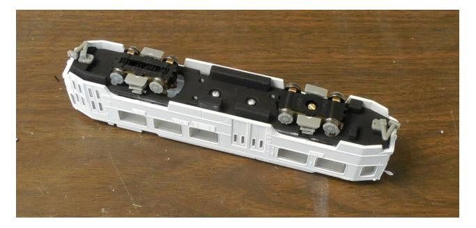
7. Install Completed and Tested Powered Frame as shown. It clips in as the original frame did. Make sure it is seated properly and the pickup wires do not interfere with the mechanics of the mounting system.
