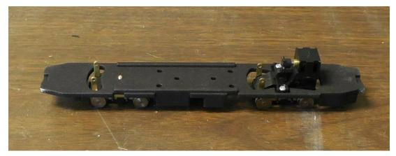
2. Install Gear and Trailer Trucks as per Bowser Instructions NOTE: On trailer truck, you can use a spring between the brass bolster screw and truck for better stability.
