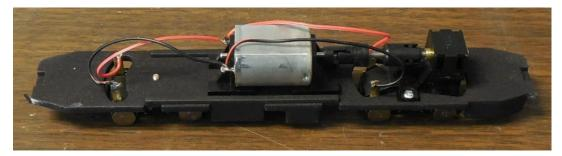
4. Install Motor on its brackets using 2-56 screws provided with the Bowser drive. Solder the wires to the motor (separate them first if they are 2-conductor, like we used) and fold down as shown to a low profile. Assemble (if necessary) and install the driveshaft. Cut the metal rod provided for it to about 11/16" (15mm) long. Lubricate bearings and gears and give it a test-run.
