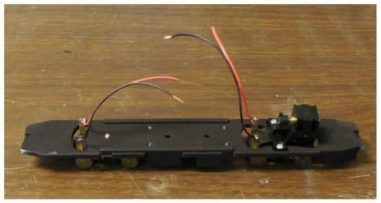
3. Solder pickup wires to brass contacts on trucks. Take care not to let the iron touch the plastic trucks or frame. Use flexible stranded wire. We used Model Power 2-conductor wire. Black on the right side, red on the left side. Length of Front wires: 4.5" (90mm) Length of Rear wires: 3" (75mm)
